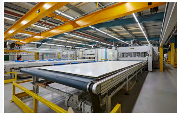
'SMART' GRP sidewall during the production process.
