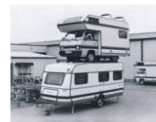
The innovative PUAL body shell is developed and proves its stability.
