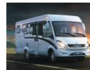
A further milestone: the Hypermobil ML-I – an integrated motorhome on a Mercedes-Benz chassis weighing less than 3.5 tons.
